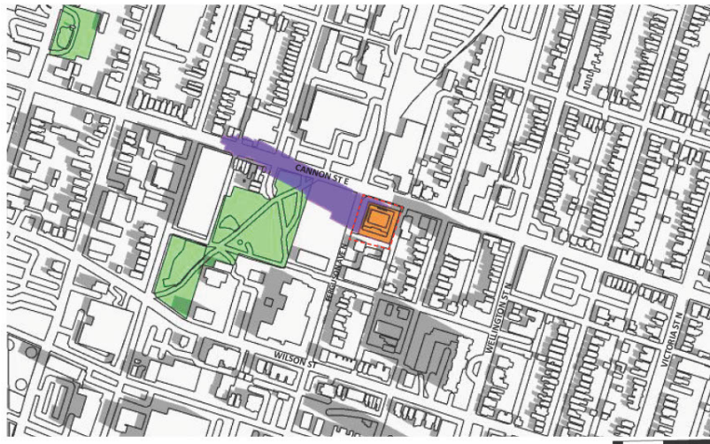
MARCH 21 st 10:00am 188 CANNON ST EAST SUN SHADOW STUDY HAMILTON JANUARY 2024 SITE BOUNDARY EXISTING SHADOWS PROPOSED SITE PLAN AS OF RIGHT MASSING PROPOSED SITE SHADOWS/ NET SHADOWS AS OF RIGHT SHADOWS OVERLAPPING SHADOWS 0 50 100 ARCADIS 5
